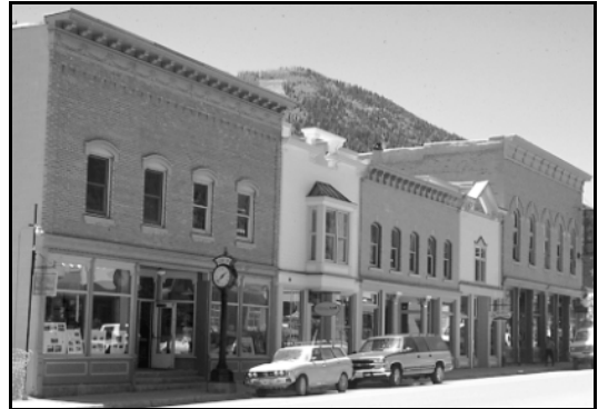
Here, a new building is divided into “modules” that reflect the traditional building widths. Contemporary interpretations of historic details are used to demonstrate that the building is new.
